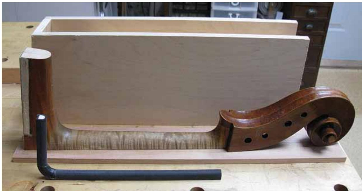
Figure 4. Carbon fiber reinforcement and routing jig.
