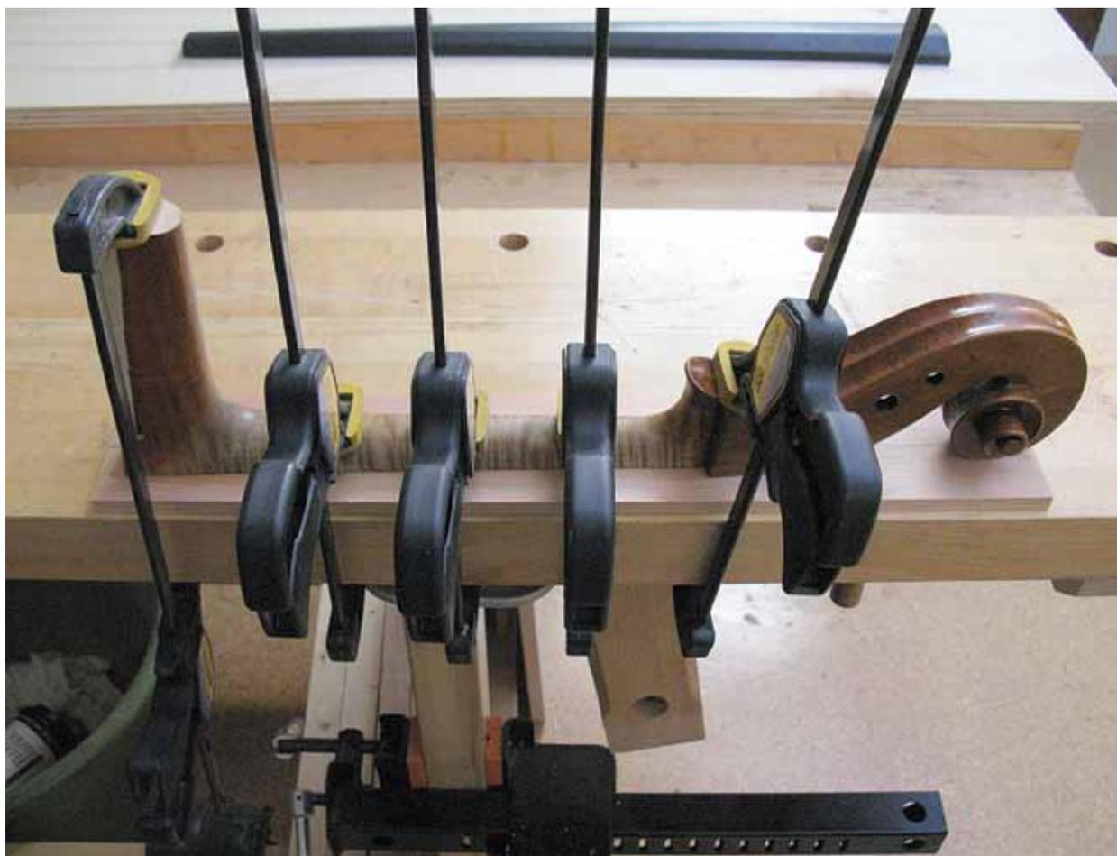
Figure 3. Gluing on sacrificial wood for routing.
