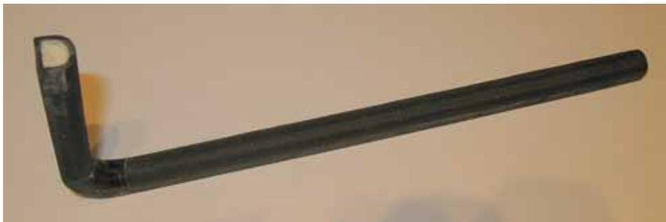
Figure 13. The carbon fiber brace.
