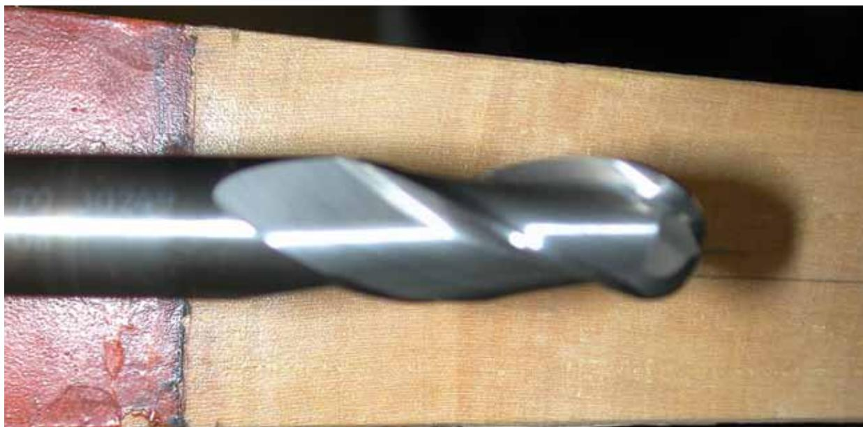
Figure 1. Three-flute ball-end cutter.
