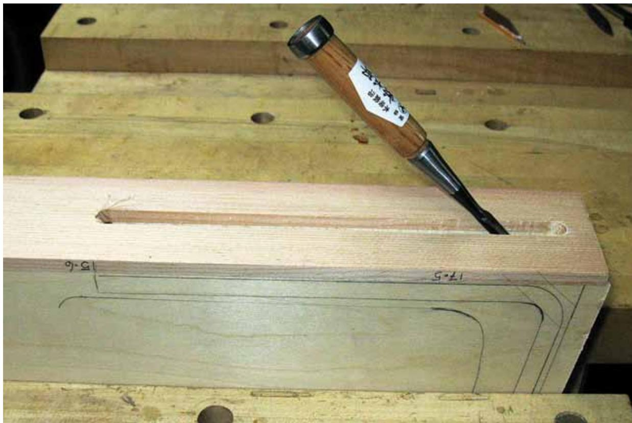
Figure 8. Gouge for the curved section.
