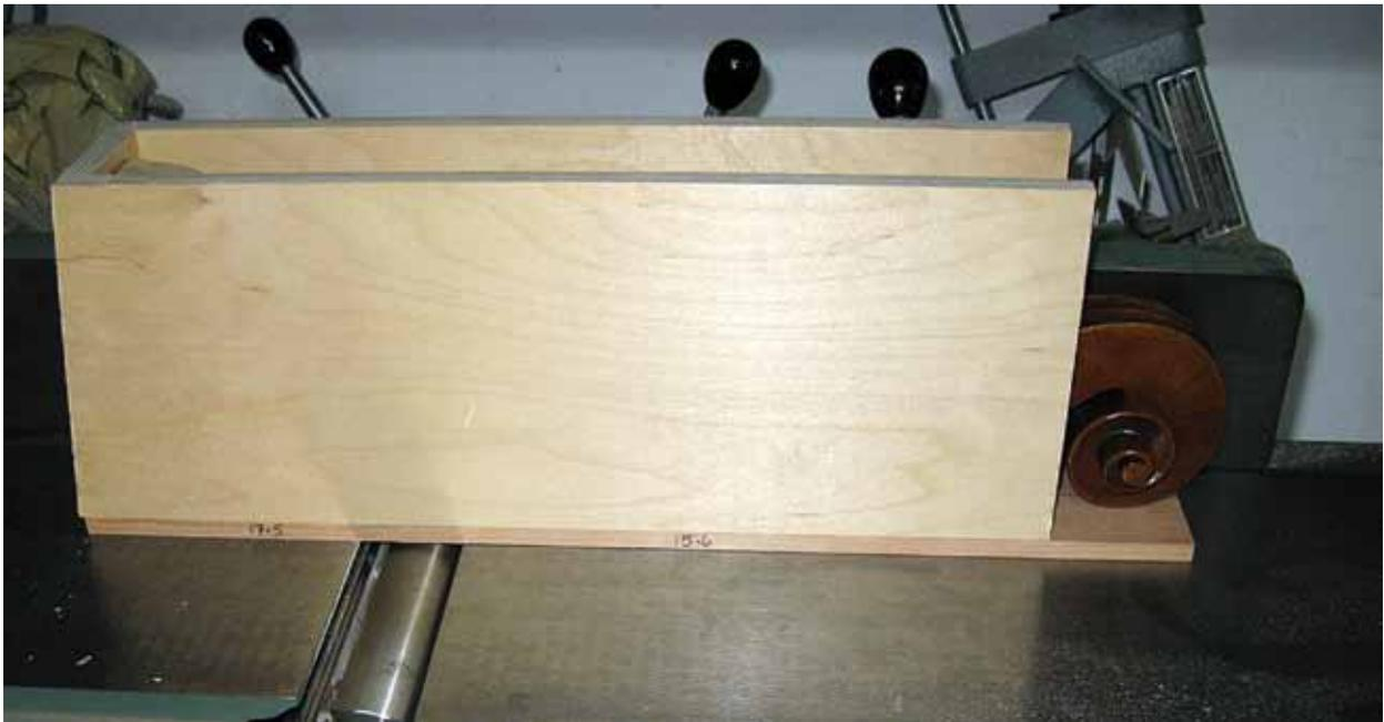
Figure 5. Jointing sacrificial surface, square to the neck heel.
