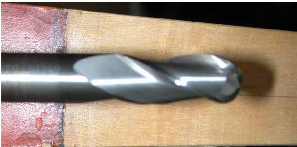
Figure 1. Three-flute ball-end cutter.
