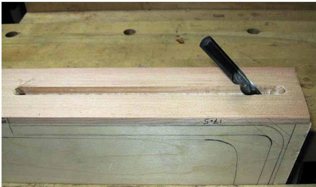
Figure 9. Drill for the curved section.
