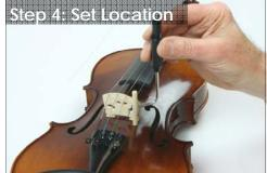
Hold the sound post setter vertically over the instrument with the sound post over the setting location and the tube of the setter over the f-hole. Loosen the sound post slightly and rotate the sound post in the setter so the angles on the top and bottom match the curvature of the top and back. Re-tighten the sound post. Note the position of the setter as this will be the position you will match when setting the post.
