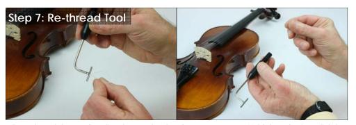
To re-thread the confiner line, loosen the thumb screw 2-3 turns. Hold the tube in a slightly downward position and thread the free end of the line into the empty hole and push through the body of the sound post setting tool.
