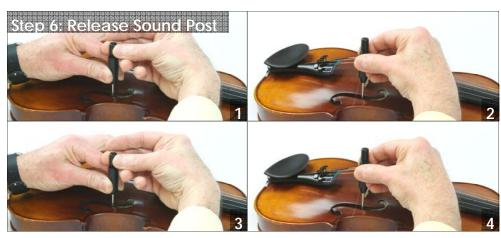
When the sound post is securely in position between the top and back, loosen the thumb screw and capture one free end of the line. Gently remove the sound post setter from the instrument. One line will pull free from the setter and release the sound post.
