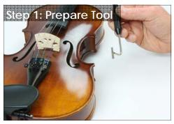
Check to see that both ends of the confiner line are threaded through the setter forming a loop around the sound post saddle. Loosen the thumb screw to allow the line to move freely.
