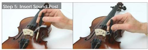
With the sound post now securely in the setter, carefully insert the sound post and setter through the f-hole and work the sound post into position holding it vertically and gently pulling the sound post towards you until you feel it wedge into position.
