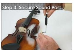
Pull the line to tighten it around the sound post and tighten the thumb screw snugly to hold it in place.
