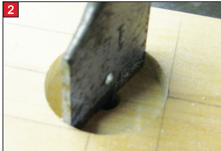
End of slot being drilled with one of my ancient spade bits. This is sized to accommodate the router guide diameter.
