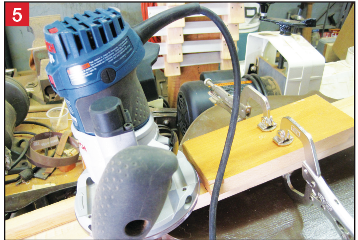
Plunge router at the end of jig with stop clamped onto the neck to limit the length of cut.
