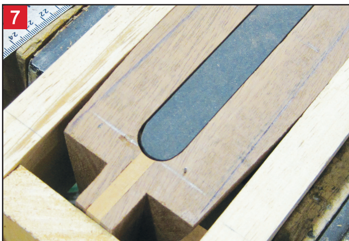
Guitar neck blank sitting in shop made router guide, dry fitted and profiled. Neck was slotted for truss rod but was filled and fitted instead with an Allred D-tube for the review.
