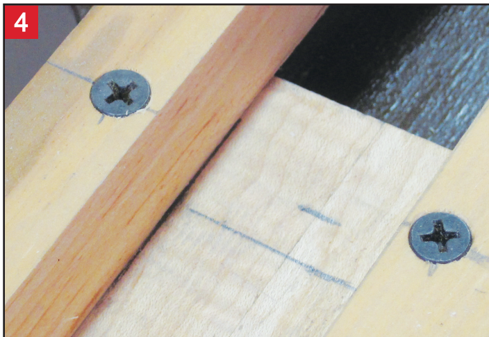
Drywall screws applying shop jig to maple bass neck, with only root-size relief holes drilled, but with no neck splitting!
